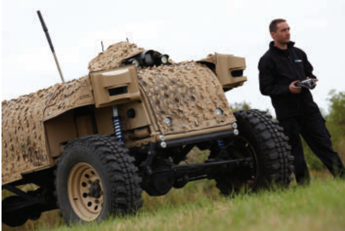
The MACE 3 unmanned ground vehicle (UGV) from MIRA features a UGV control system with tele-operational and autonomous modes.
